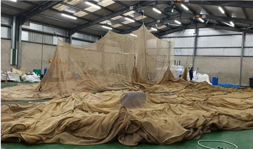
Figure 3: Salmon cage net being inspected for repair at MOWI's net recycling facility.
