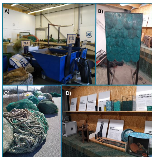
Figure 8: A) Sotenäs Marine Recycling Center (SMRC) sorting facilities; B) Plastic tiles made from recycled fishing gear at SMRC; C) Collected end-of-life and historical fishing gear at SMRC and D) Plastic pellets and prototypes made from recycled fishing gear at SMRC. Images provided by SMRC.
